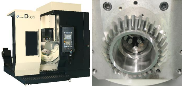
D500 ( m5, z30, \alpha20^\circ, \beta=0^\circ, d=150 ) (Provided by Makino Mill Inc.)
