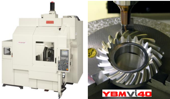
YBMvi40 ( m5, z20, \alpha20^\circ, \beta=35^\circ, d=100.0 ) (Provided by Yasuda Kogyo Co., Ltd.)
