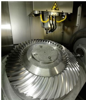
HERMLE C-50U ( m10, z47, \alpha20^\circ, \beta=35^\circ, d=470 ) (Provided by Aichi Sangyo Co., Ltd.)
